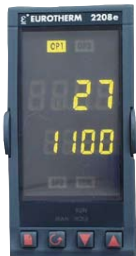
Regulator temperatury komory pieca Eurotherm 2208e
